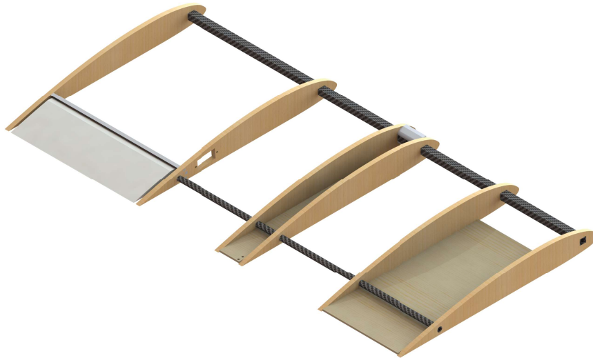
Figure 12: The initial wing structure
