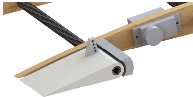
Figure 14: Cross-section of the aileron structure
